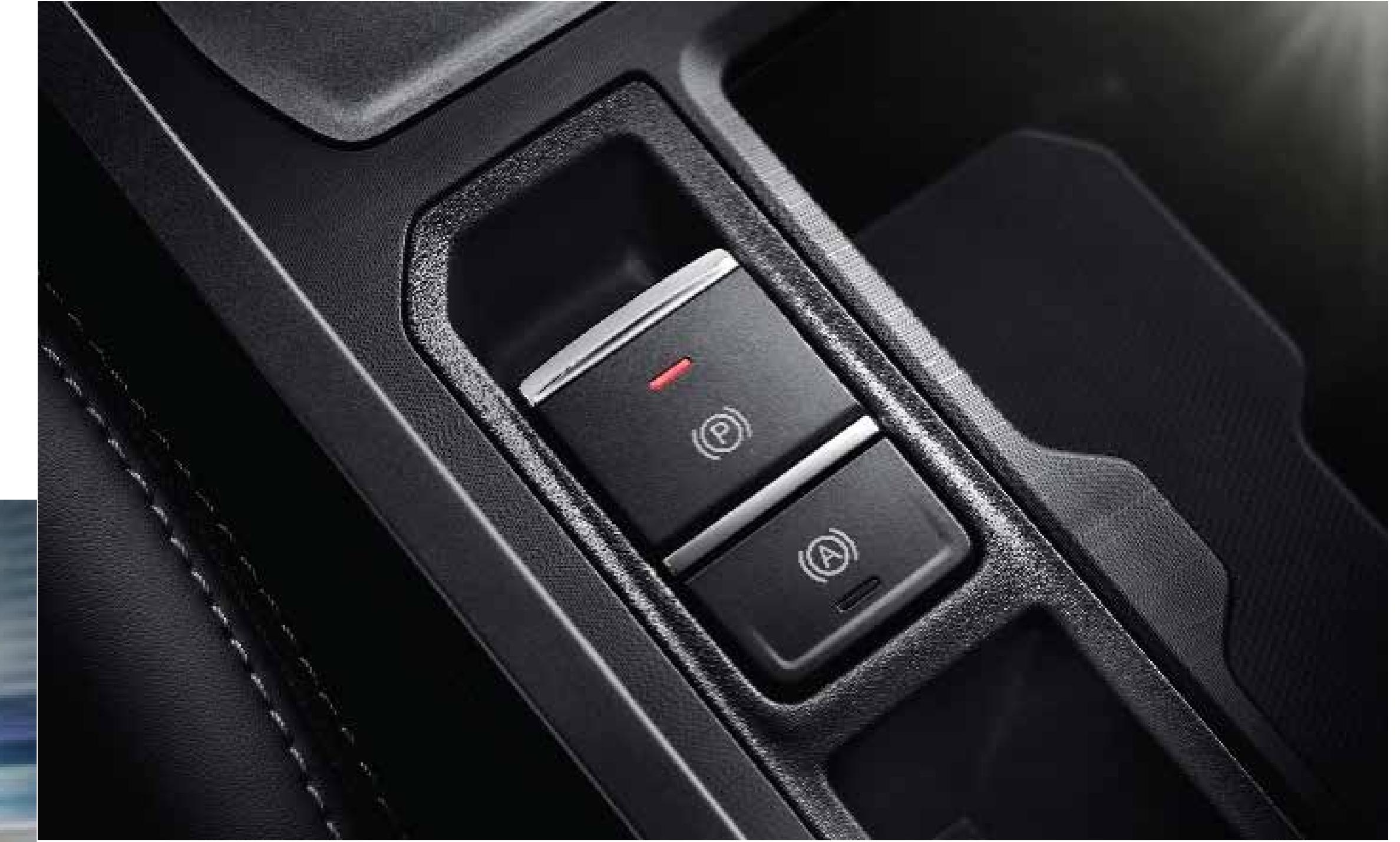
**EPB(Electric Power Braking)**
